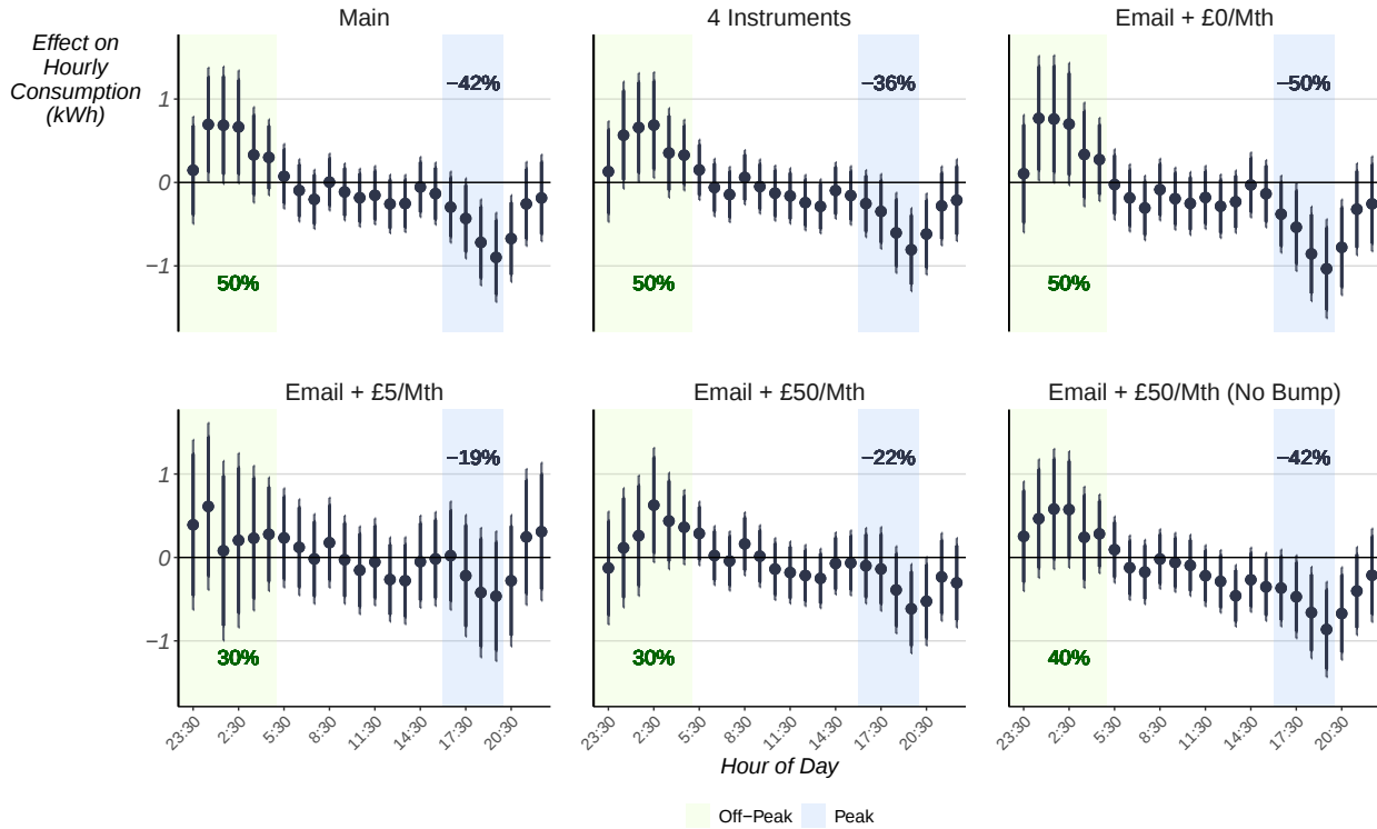
Figure 7: Impact of EV Tariff on Electricity Consumption
